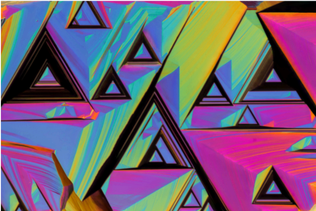
(2) This diamond from Hudson Resources, Garnet Lake in Western Greenland shows classic trigon etching on the surface of an octahedral crystal face as seen using differential interference contrast microscopy. Field of View 0.72mm, Copyright GIA. Stone courtesy of the John Koivula Inclusion Collection.
