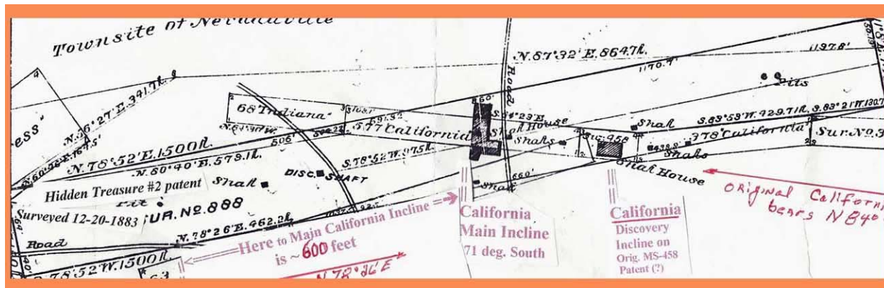
Figure 2. Plan of the California #557 claim, at center. The claim is 50 feet wide. The shaft immediately to the right (east), on discovery claim 958, followed low grade base metal ore downward.
