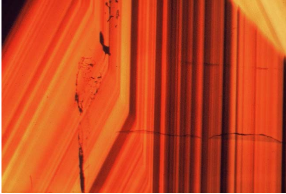
Figure 7. Transmitted plane light photomicrograph of a single gemmy orange hübnerite blade from the Coors Pocket. Note the compositional banding. Gemmy orange bands are essentially pure MnWO_4 . Only a very small amount of iron (<0.35 wt. %) substituting for the Mn is required to turn the orange hübnerite into the black bands. Horizontal field of view is 1.05 mm. Photo by Karen Wenrich.
