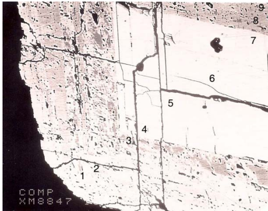
Figure 11. Cherry rhodochrosite is transparent in thin section whereas the lower-quality pink rhodochrosite forms rims and fills fractures that are dark and cloudy. Electron backscatter image; horizontal field of view is 250 \mu m. A traverse of spot chemical analyses was made across this sample, providing an excellent demonstration of the substantial variation in Fe, Ca, and Mg content between the cherry and pink rhodochrosite. The spots are recorded by number on the photograph and correspond to the sample numbers in the following table of Fe, Ca, and Mg contents in weight percent. Note the low Fe content for spots 4-7 and the associated clear purity in the backscatter image.
