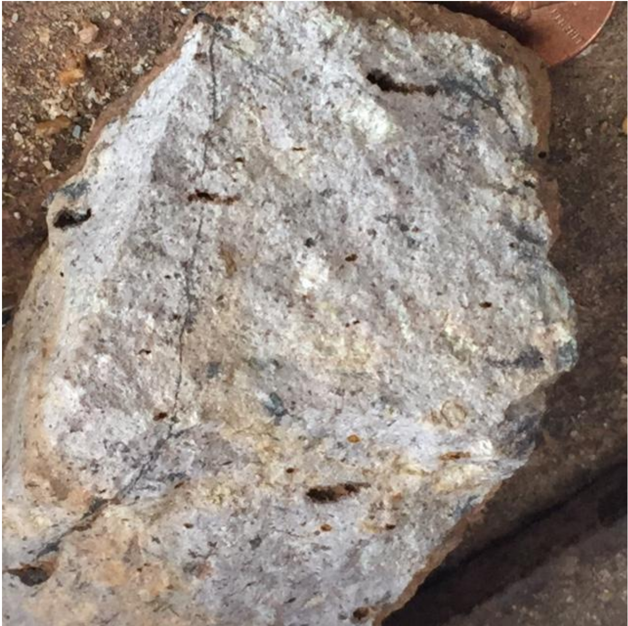
Figure 12. Vuggy bostonite from shaft (dump) that produced from Hidden Treasure vein, northwesterly slope of Quartz Hill. This is probably the California dike (Sims et al., 1963 plate 1). Lilac with beige oxidation fronts, very fine grained, equal granular, vesicular, with secondary rusty brown Fe oxide stained quartz lining vugs up to 3-6 mm, with oxidized sulfides, and occasional clots of fine grained pyrite. 1 % 1mm anhedral - euhedral quartz phenocrysts occur sporadically throughout sample in groups. <1 % 3-4 mm Clay altered K feldspar subhedral phenocrysts are found with trachoidal alignment. Minor anhedral epidote green phenocrysts, plagioclase altered to sericite. Trace pyrite blebs <0.5 mm disseminated in ground mass. Hairline Quartz veins with minor fine galena salvages.
