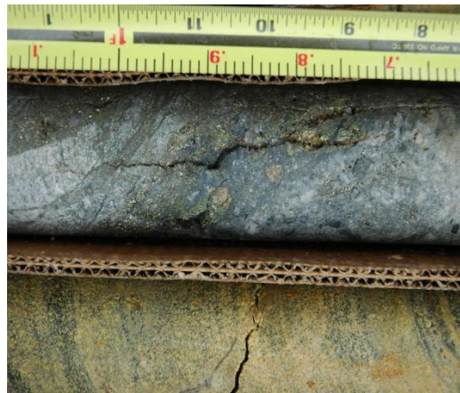
Figure 6:. Foot & Simmons Vein, Main Stage Composite Sulfide Vein, fractured coarse chalcopyrite grains surrounded by tennantite, 0.183 oz/t Au, 1.78 oz/t Ag, 1.58% Cu, BH0602, 388.2-389.2 ft.
