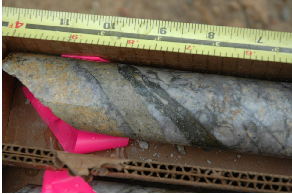
Figure 9. Hartford Vein, hessite (?) silver telluride vein adjacent to fragmental tan chalcedony vein, 0.028 oz/t Au, 2.27 oz/t Ag, 0.4% Cu, 24 ppm Te) BH0707, 1655.5-1656. Ft.
