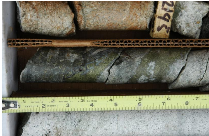
Figure 5. Buell (UPR) Vein at -1300 ft. (-396 m) depth, Main Stage Composite Sulfide Vein, fractured coarse chalcopyrite grains surrounded by tennantite stockwork, 9.21 oz/t Au, 6.3 oz/t Ag and 3.43 oz/t Au, 5.37 oz/t Ag, 4.48% Cu, BH07-08, 2147 ft.
