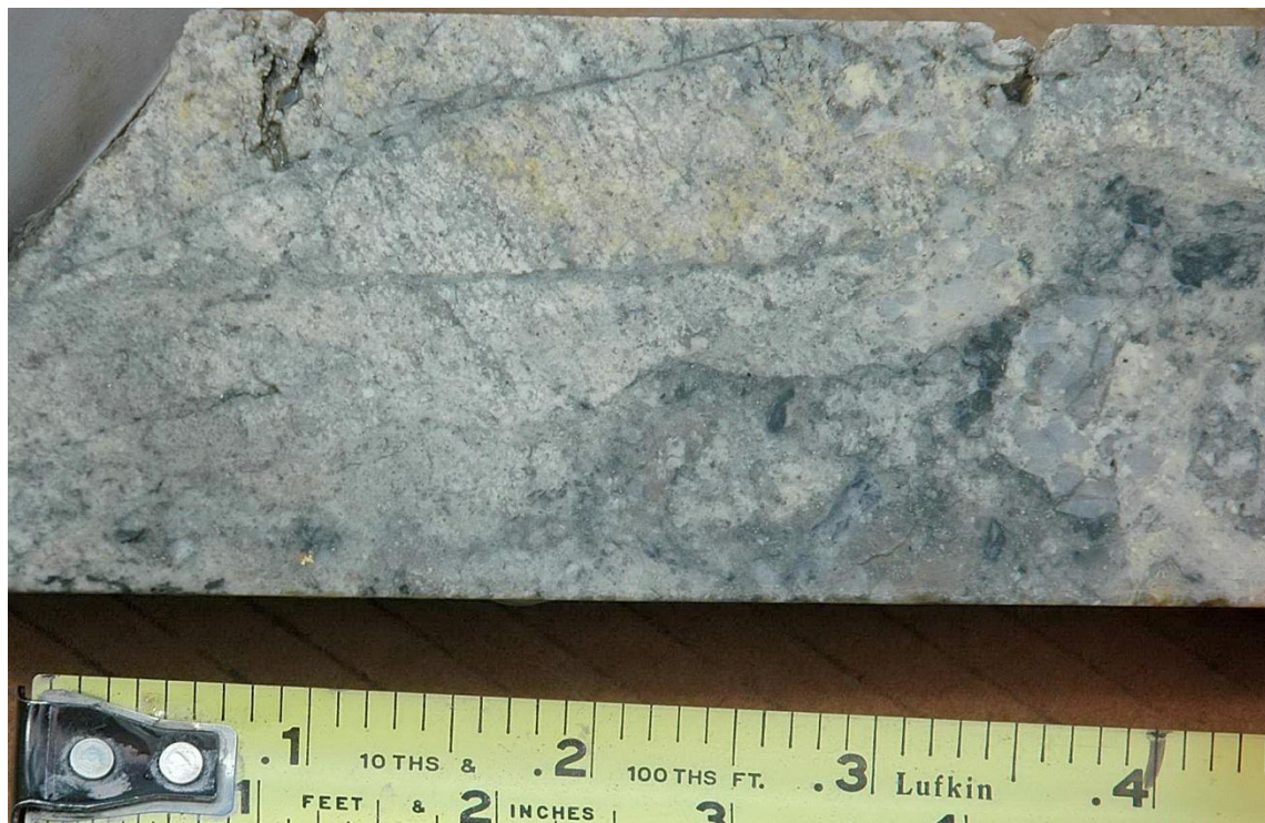
Figure 8. Shattered Pegmatite Breccia, Cousin Jack Vein, 0.75 oz/t Au, 0.28 oz/t Ag, 0.02% Cu, 5 ppm Te BH08-09, 501.5-503.5 ft.
