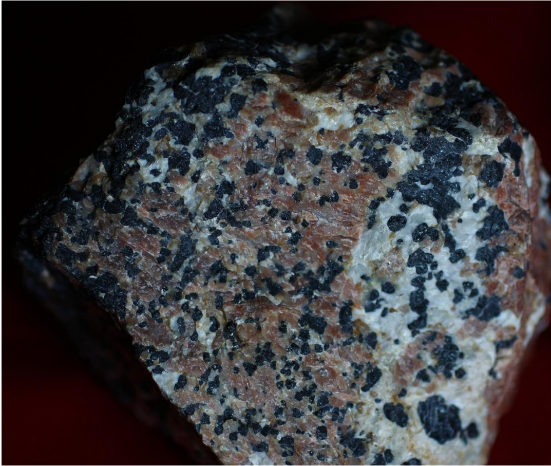
Figure 14. Typical Sterling Hill ore sample, consisting of willemite (pinkish brown), franklinite (black), and calcite (white), from the 1400 level, Sterling mine. Sample is 10 cm across. (Carnein specimen and photo)
